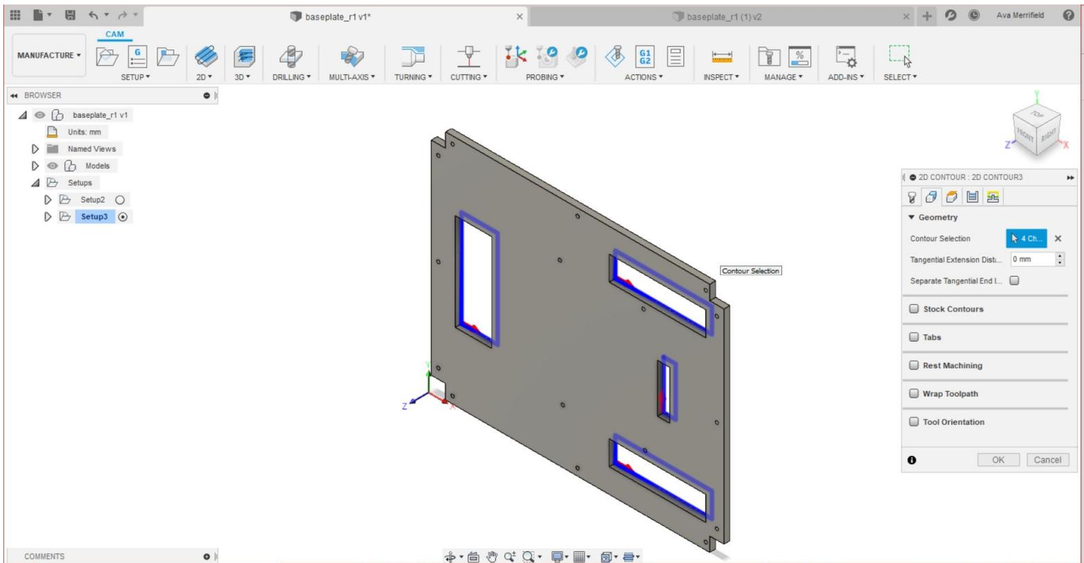
2. In the contour menu, go down to where it says “Multiple Depths” and select it. This means the CNC will make multiple passes as it cuts, rather than try and cut all the way through the material the first time. Select “Okay”.
