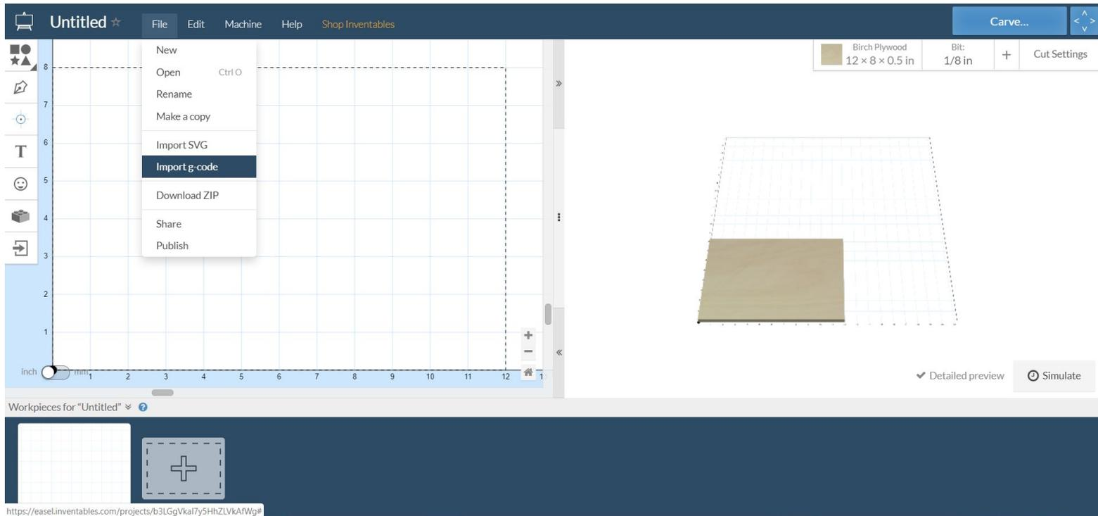
5. In Easel, click on “File” and select “Import G-Code”. Click on the file in your output folder that you want to cut. Your part should appear on the grid. Make sure it’s set up the same way you have it set up on the wastebard.
